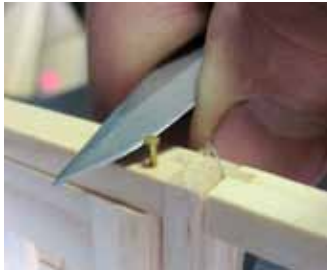
Door: remove the pins
