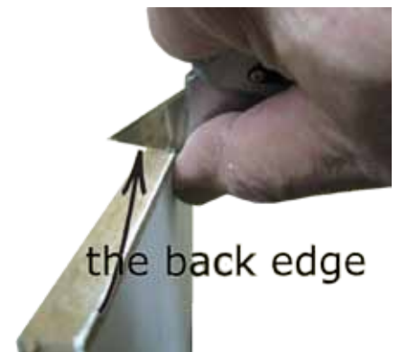
Cleaning an edge with the back of a utility knife blade
