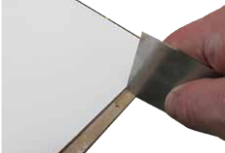
Cleaning a groove with a Cabinet Scraper
