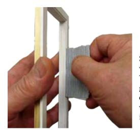
Sanding after the first coat is what makes the wood smooth. The paint fills and stabilizes the grain, so the sandpaper can clip off the roughness and leave the wood silky and uniform. Sand in all the corners and details.
