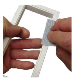
3. Sand after the first coat until the wood is smooth and the paint is transparent.
