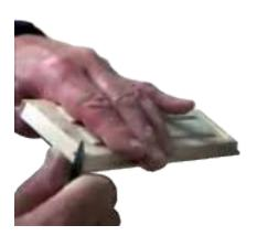
1. Pull the bottom Pin with a knife. Tip the Door out - pull the top pin with plyers.
