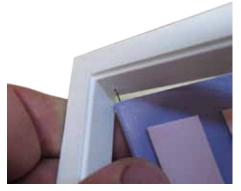
7. Feed the Top Pin into the hole in the door top frame
