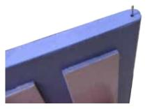
5. Put the headless pin in the top hole
