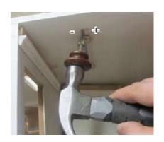
Eyelet the ExtraBrite LED to the Tapewire, "+" to the copper and "-" to Blue.
