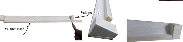
Glue Valance Ends to each end of the Valance Front. The sloped face of the Valance End is the Front. Mark and cut the Valance Base to fit between the Ends.
