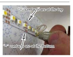
Punch a hole in a "+" contact and a "-" contact. Remember the first photo? The blue lead ("-" in this house) was toward the back. So the back wire is going to the "-" side of the ExtraBrite© Striplight, which is at the bottom here. Insert the wire and secure with an eyelet (don't hit the emitter with the end of the tool).
