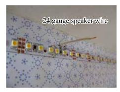
Strip both ends of a short piece of wire. Poke an end into the hole.
